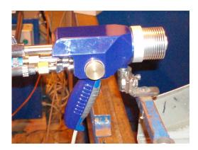
MOGUL Hi-Speed is a High-Velocity-Oxygen-Fuel thermal spray equipment.
