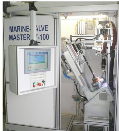
Plasma-Transfer-Arc Welding is a process where a powder is hard-faced to a substrate using a transferred plasma arc. Big advantage is that dilution is very low and can be controlled.
