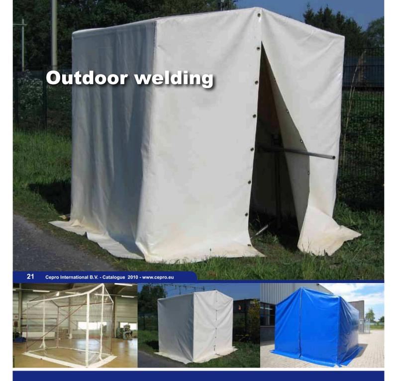
This standard tent has a width of 1900 mm, a depth of 2000 mm, a height of 2000 mm at the sides and 2200 mm in the middle. The cover is made from a white PVC fabric and is self-extinguishing according to the French standard M2. The weight of the fabric is 590 grams per square meter. The tent can be closed at both the front and the back. The tent is fitted with 200 mm wide ground flaps all around. The tent comes with a frams  $\varnothing$  25 mm galvanized tube frame.
