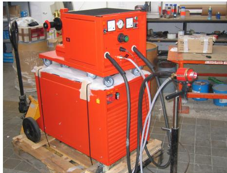
MOGUL A 4P is a modern, high-performance arc spray equipment for manual and/or automatic operation.
