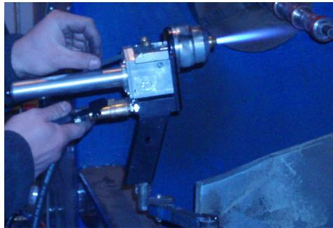
Excellent ceramic coatings for wear and corrosion resistance, electrical insulation and thermal barrier application are achieved by the MOGUL OX-E rod spray system.
