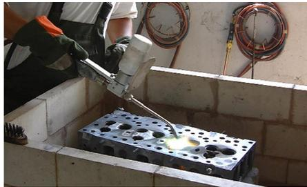
The MOGUL XS 7 is a powder fuse welder using acetylene and oxygen (no air required). The XS 7 grip can also be used for brazing and cutting torches (options) and further more can be used as a simple thermal-spray gun especially for powders which are going to be fused after spraying (MOGUL XS 4 respective MOGUL XS 8).
