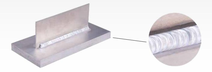
Welding of diverse thikness sheets: The concentration of the energy transfered to the workpiece allows the
