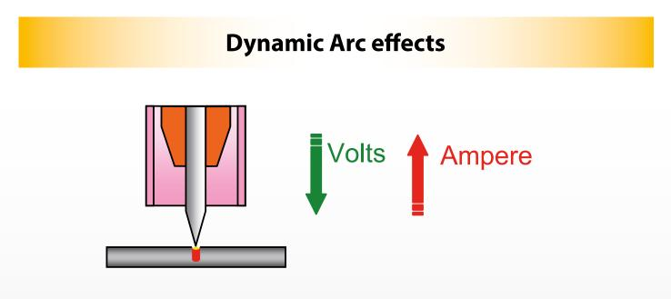
The Dynamic Arc function permitts the welding with extremely short arcs. When the electrode is very close to the base material, the current increase avoids the contact by the shifting of the welding pool. This prevents both the electrode's sticking at the material and the inclusion of tungsten's particles on the deposit.
