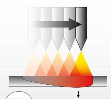
The continuous welding current supplies a continuous energy that prevents the workpiece cooling and causes its overheating with consequent excessive penetration and deformation.
