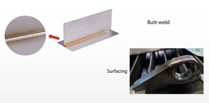
In the fillet welding it is possible the use of Multitack which allows to achieve excellent results. The weld remains white and without any oxidation, thus prevents the acid treatments which often must be applied post welding.
