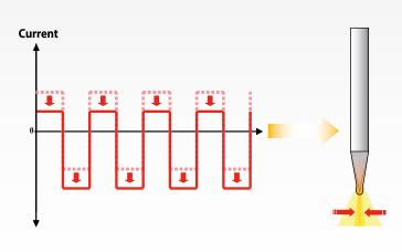
Thus function makes it possible to shift the waveform towards the negative part with respect to zero. This makes it possible to create a highly penetrative and precise fusion bath so that very light gauge sheets can be welded with an electrode tip comparable to that of an electrode for DC - TIG welding. The adjustable value in our AC/DC TIG power sources ranges from 0% to 80% (with respect to the DC half-wave percentage).
