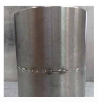
Pipe weld application 5/4 x 2mm
