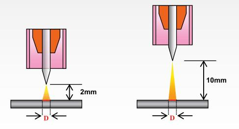
When the arc length changes, the melting pool maintains exactly the same width (D) avoiding the base material's overheating, any plastic deformation and any loss of its mechanical features.
