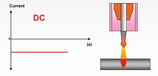
During the TIG DC half period there is high penetration in the workpiece.
