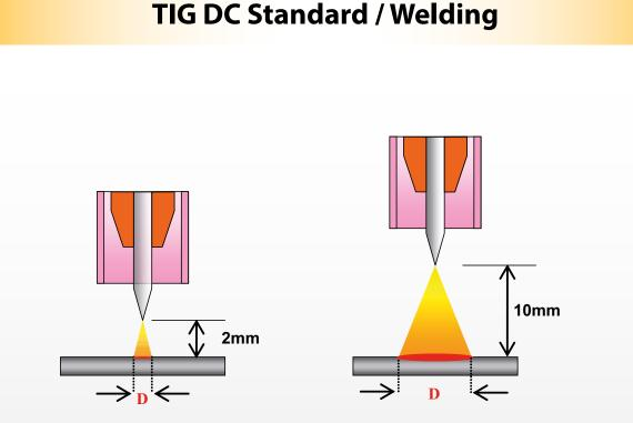
When the arc length changes, the melting pool (D) becomes wider with consequent increase of the heat output on the base material which is subjected to overheating.
