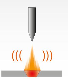
The Q-START (Quick Start) function makes it possible to minimise sheet tacking. A series of adjustable duration pulses creates a movement of molten material between the two edges in order to accelerate the join. This function is invaluable in the case of seams with slight openings or with irregular preparation.
