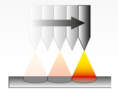
The series of repeated arc strikes at short time intervals allows the material to cool during the pause between one strike and the next.
